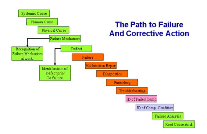
As described above, any failure event typically begins with a Systemic Cause. The Systemic Cause creates a "trap" into which an individual can fall. The next step is the Human Cause in which a specific individual either does something or fails to do something that produces a Physical Cause. The third step is the Physical Cause. This is the step in which the form of prevention used to restrain natures Failure Mechanisms are ignored.
